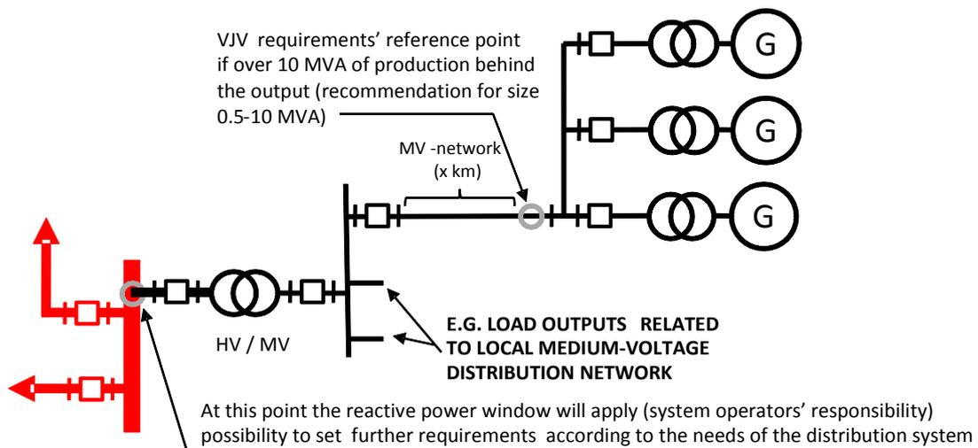
**Figure 6.3** The point where the requirement set for the reactive power production capacity must be met with respect to a power plant formed by several generators and a generation unit
