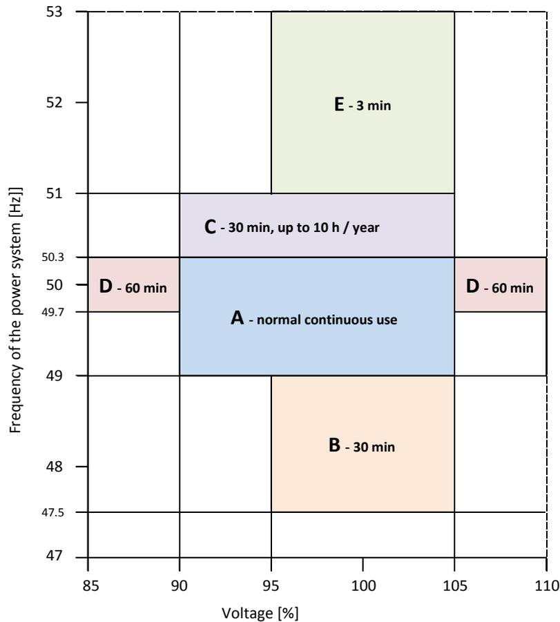
**A:** Normal continuous use – reduction in the production ability of active and reactive power due to the voltage and/or frequency of the power system is not permitted
