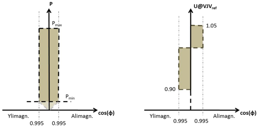
**Figure 6.4** The requirement for reactive power capacity set for the generation installation.  $U@VJV_{\text{ref}}$  refers to the voltage in the reference point defined in Fingrid Oyj's technical requirements for the power system (VJV).
