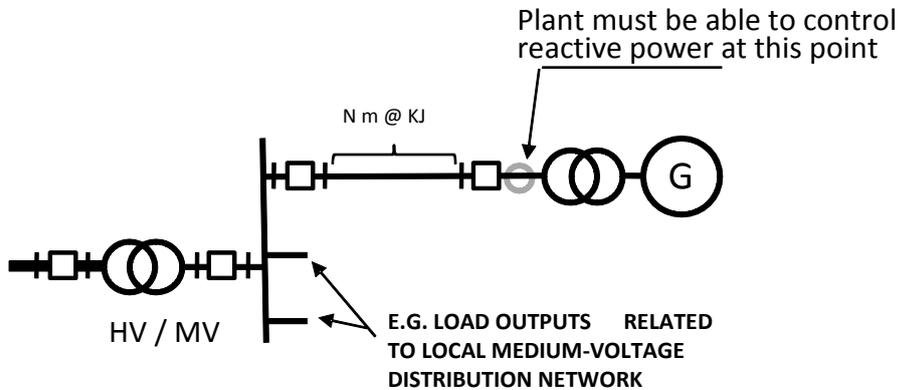
**Figure 6.2** The point where the requirement set for the reactive power production capacity must be met with respect to a power plant formed by an individual generator and a generation unit
